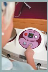
Position **Rubis** at the end of the bed and select temperature. Press the heater button and wait for **Rubis** to reach desired temperature (this takes approximately ten minutes from cold)
